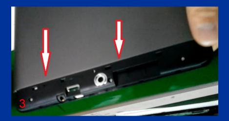
Maintenance Steps 2 Remove the backshell
