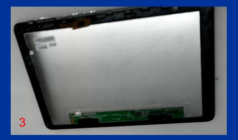
Maintenance Steps ④ Remove the LCD screen
