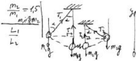
$$\begin{cases} m_1 v_1 = m_2 v_2 & (3C) \text{ ②} \\ m_1 \frac{v_1^2}{2} + \frac{m_2 v_2^2}{2} = m_1 g h_1 + m_2 g h_2 & (3C) \text{ ③} \\ \cos \alpha = \frac{L_1 - h_1}{L_1} & \text{①} \\ \cos \alpha = \frac{L_2 - h_2}{L_2} & \text{②} \\ -m_1 g + T \cos \alpha = m_1 a_T & \text{③} \\ m_1 a_T = T \cdot \cos \alpha & \text{④} \end{cases}$$
