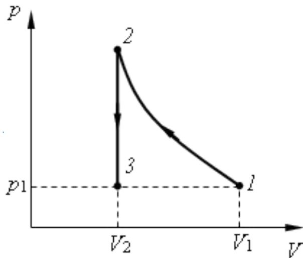
$$\Delta U = \frac{i}{2} p_1 (V_2 - V_1)$$
