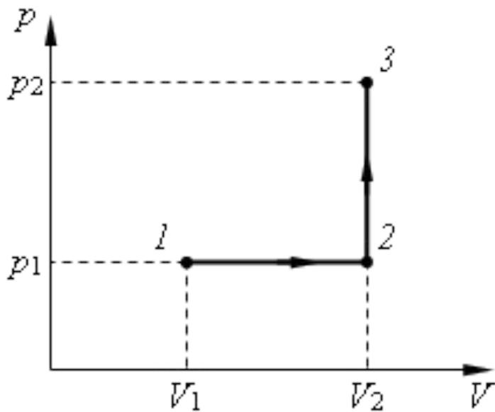
$$A = A_{12} + A_{23} \quad A_{12} = p_1 (V_2 - V_1) = 2p_1 V_1 \quad A_{23} = 0$$
