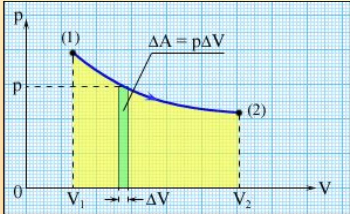
$$A = \sum_{n=1}^N p_n \Delta V = \int_{V_1}^{V_2} p dV$$
