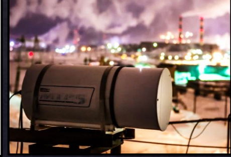
MTP-5 microwave temperature profiler (Norilsk only)
