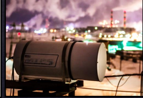
MTP-5 microwave temperature profiler (Norilsk only)
