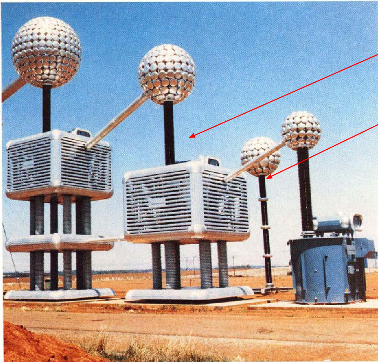
Three-stage cascade transformer 3 \times 600 kV, 2 A cont. outdoor type with AC voltage divider 1500 kV
