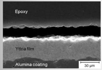
SEM micrograph of sample 3; high magnification showing the alumina coating and yttria film.
