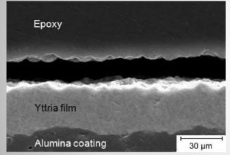
SEM micrograph of sample 3; high magnification showing the alumina coating and yttria film.
