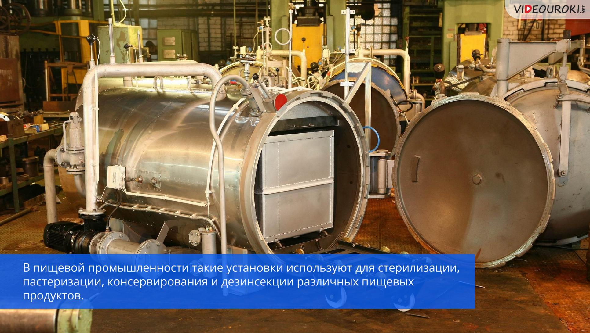
A row of industrial stainless steel autoclaves in a factory setting. The foreground unit has its circular door open, revealing a metal tray inside. The background shows more similar units and factory equipment.
