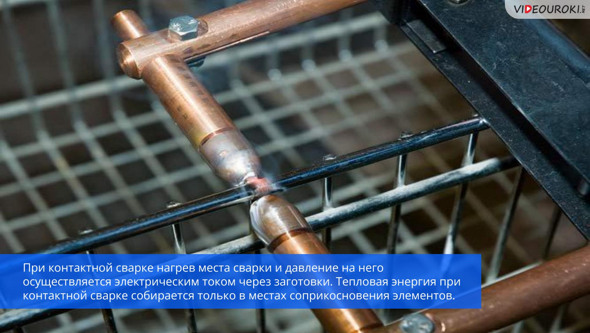
A close-up photograph showing the contact welding process. Two copper rods are being joined together. A bright, glowing point of contact is visible where the two rods meet, indicating the heat generated by the electric current. The rods are held in place by a metal frame with a grid pattern in the background. The lighting is focused on the welding point, creating a high-contrast scene.
