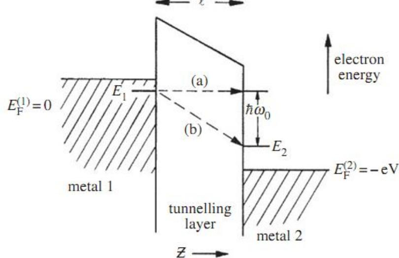
**Figure 5.** Lambe & Jacklevic demonstrate inelastic electron tunnelling through a metal junction, from [32]. There are two possible ways for the electron to cross the tunnelling layer (insulating barrier) via (a) an elastic or (b) an inelastic transition. The inelastic transition occurs when there is a molecule bridging the tunnelling layer with a mode of vibration,  $\hbar\omega_0$ , that the tunnelling electrons excites, and so loses energy too.
