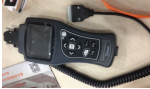
ZAPI handheld programmer, model CAN smart console
