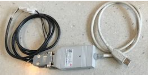
CURTIS PCAN for modification of parameters for lithium battery
