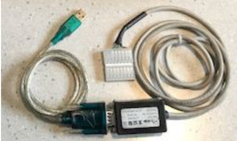
ZAPI program downloading cable, model SCH INTERFACCIA PC/ADAPTER
