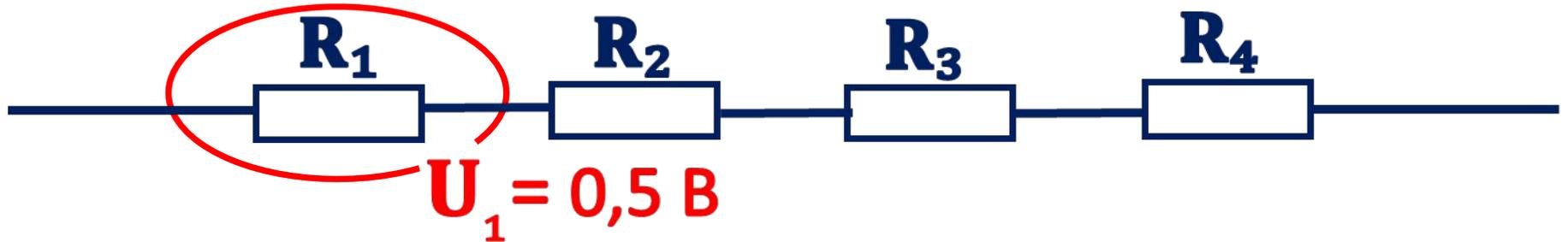
$$\mathbf{J_1 = \frac{U_1}{R_1}} \quad \mathbf{J_1 = \frac{0,5\text{ B}}{1\ \Omega} = 0,5\text{ A}}$$
