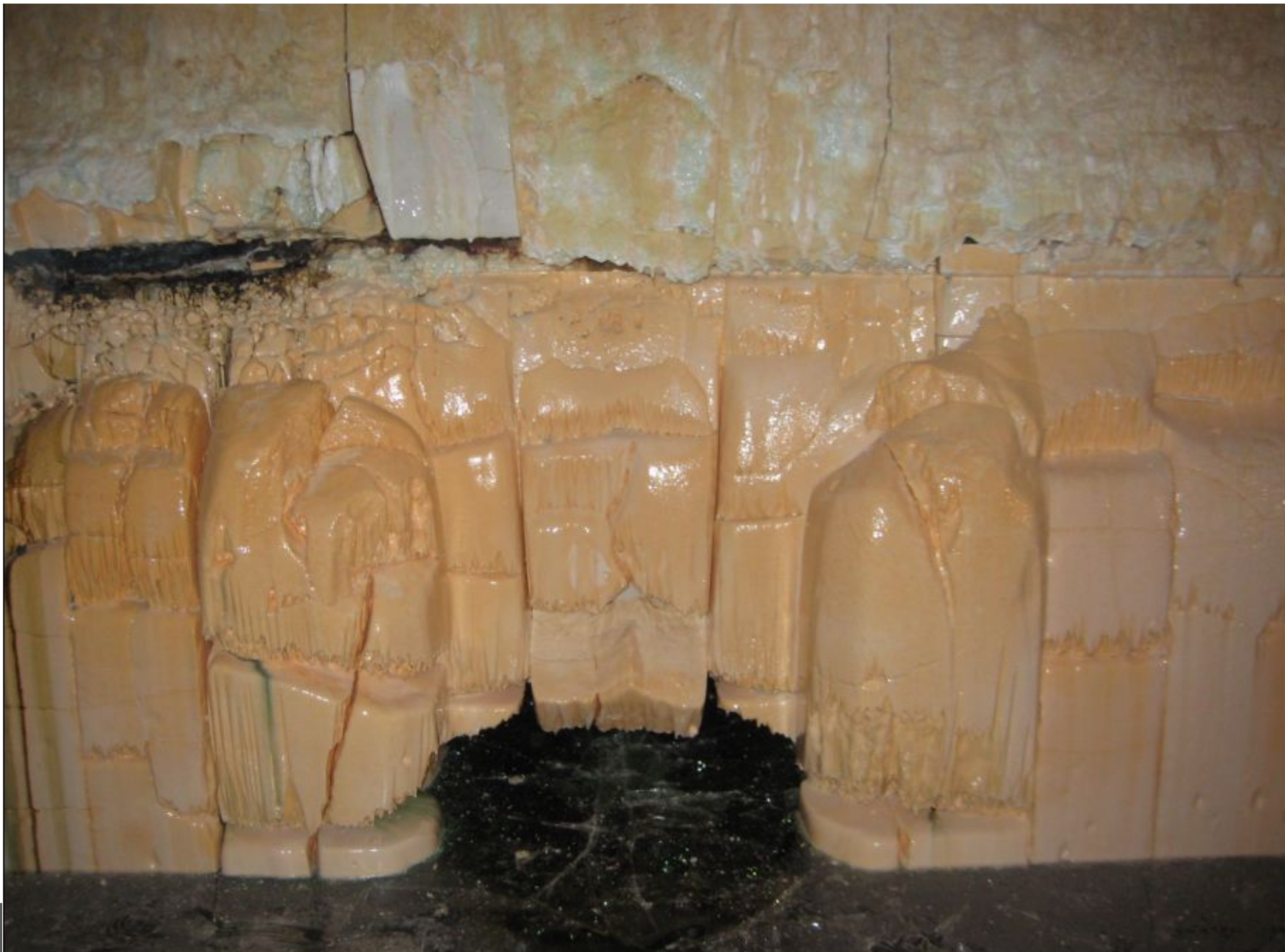
Throat angle blocks after 5 years campaign with insufficient air cooling
