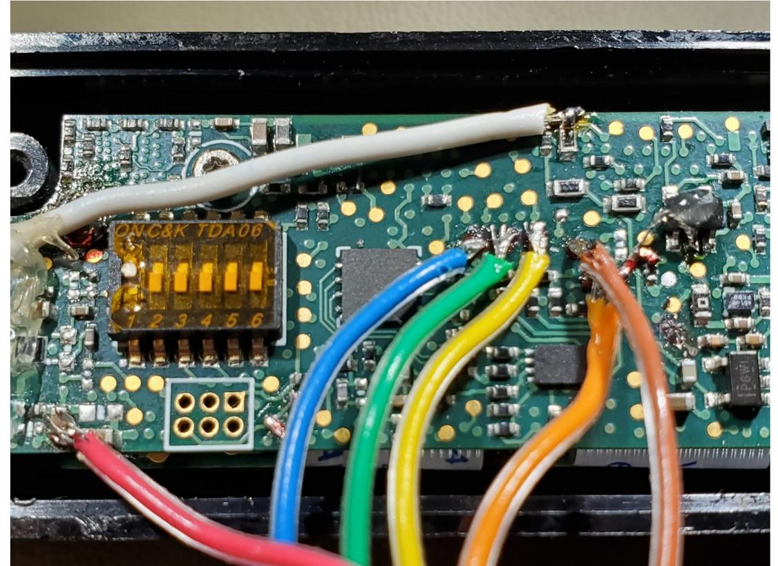
Fig.5 – Connector soldered
