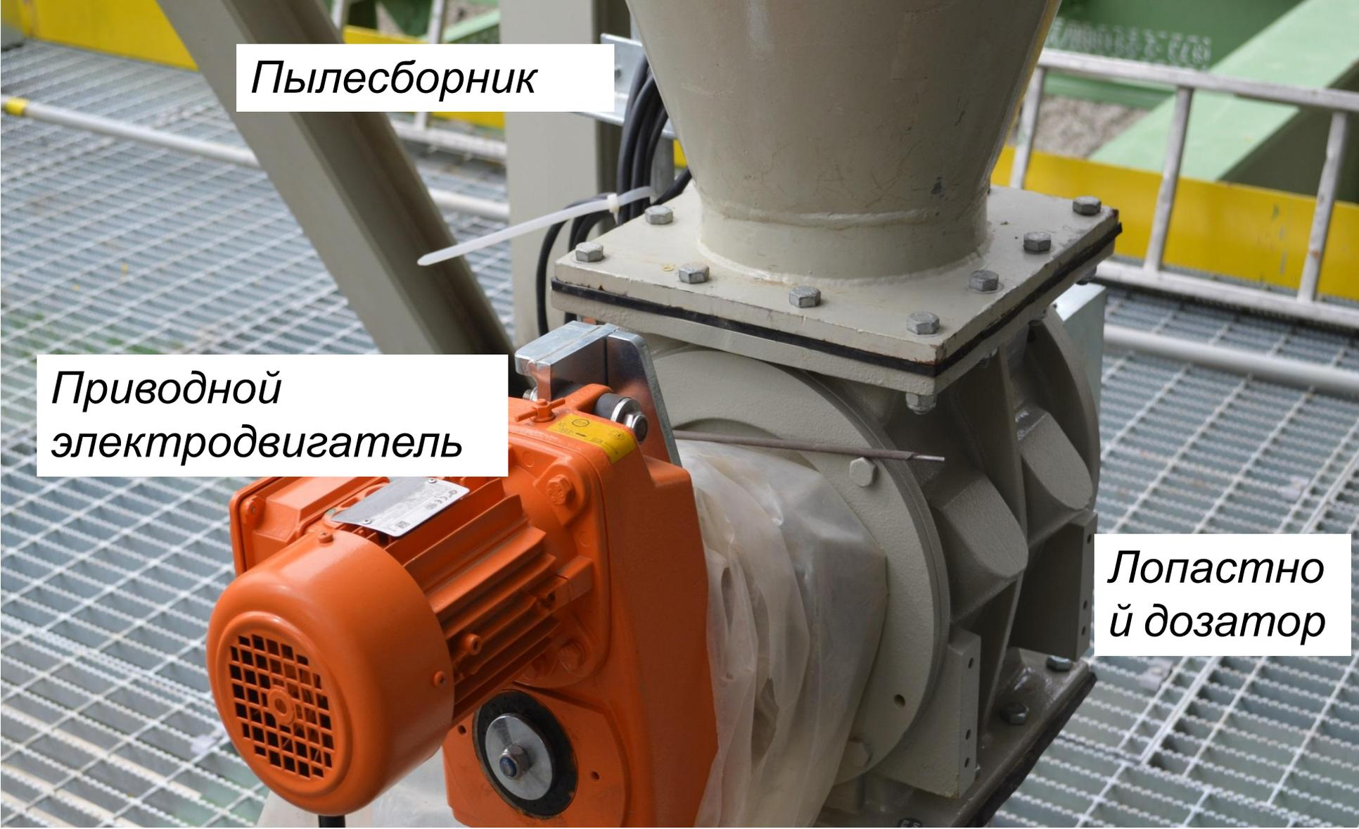
A close-up photograph of an industrial dust collector. The main body is a light grey, conical hopper. At the bottom, it is connected to a white, lobe-shaped doser. An orange electric motor is mounted on the side of the doser. The entire unit is mounted on a grey metal grating floor. In the background, there is a yellow and white safety railing.
