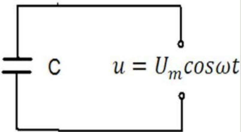
$$u = \varphi_1 - \varphi_2 = \frac{q}{C} \quad \frac{q}{C} = U_m \cos \omega t. \quad q = CU_m \cos \omega t$$
