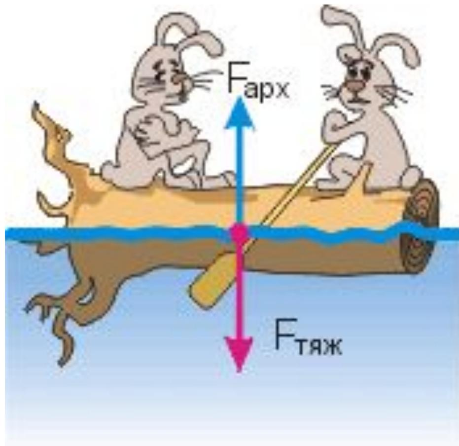
$$F_{\text{Арх}} = P_{\text{ж/г}} = g \cdot \rho_{\text{ж/г}} \cdot V_{\text{т}}$$
