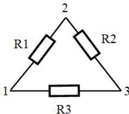
$$\begin{cases} R_{12} = \frac{R1(R2 + R3)}{R1 + R2 + R3}; \\ R_{23} = \frac{R2(R1 + R3)}{R1 + R2 + R3}; \\ R_{31} = \frac{R3(R1 + R2)}{R1 + R2 + R3}. \end{cases}$$
