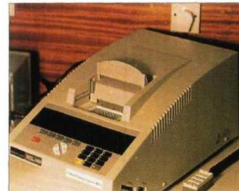
81 Thermal cycler used in the polymerase chain reaction.
