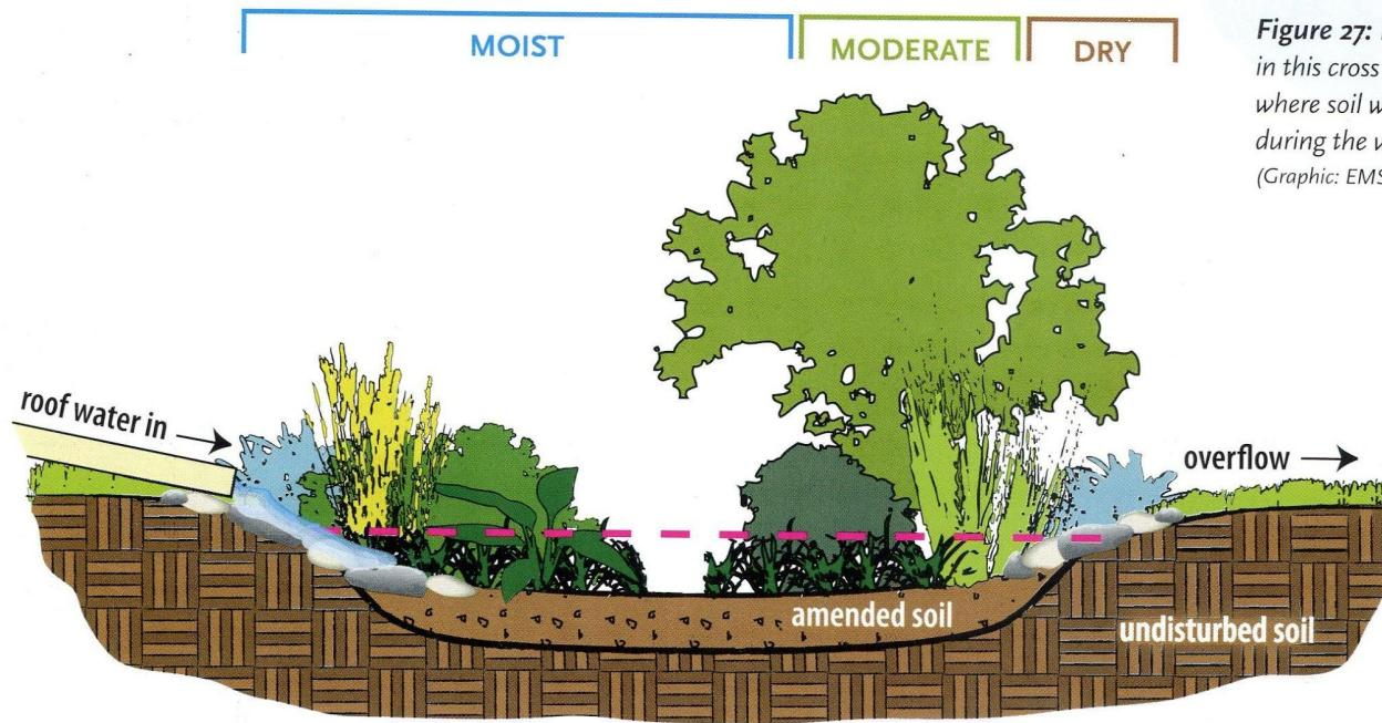
Figure 27: Planting zones in this cross section illustrate where soil will be moist during the wet season.
