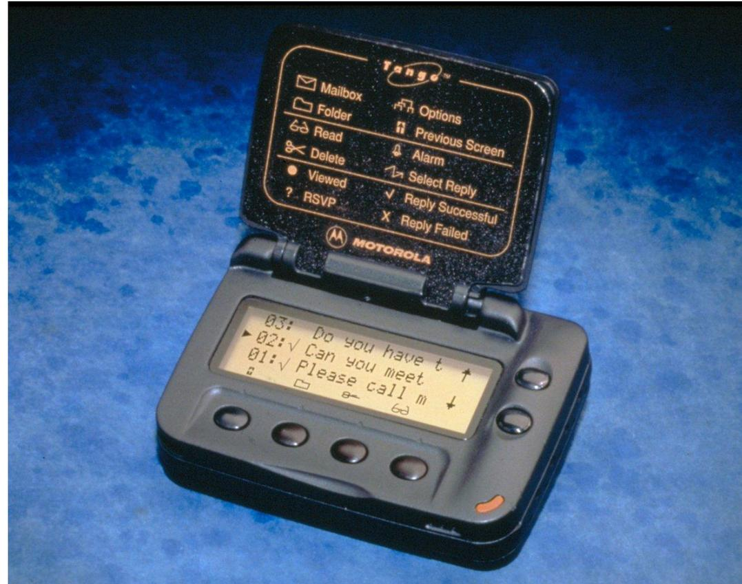
1995: Motorola introduced the world's first two-way pager, the Tango two-way personal messaging pager. It allowed users to receive text messages and e-mail, and reply with a standard response. It also could be connected to a computer to download long messages.
