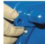
Once adjustments have been made, the unique lock collar and adjusting screw maintains the clearance setting even if the coverplate is removed.
