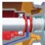
A patented atmospheric isolation barrier, along with two lip seals provides maximum bearing protection. This unique design also provides for external monitoring.
