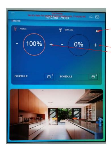
Scheduling On/Off button, orange color to reflect status where Orange means On and white means Off. This button should enable to device to run in schedule or manual. When ON the device should run as per the schedule set, when Off the device should run as per the command given from the app
