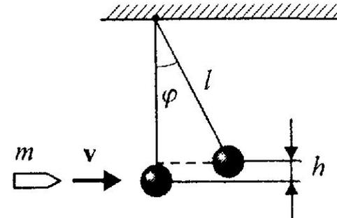
$$\varphi = \arccos \left[ 1 - \frac{(mv)^2}{2gl(m + M)^2} \right]$$
