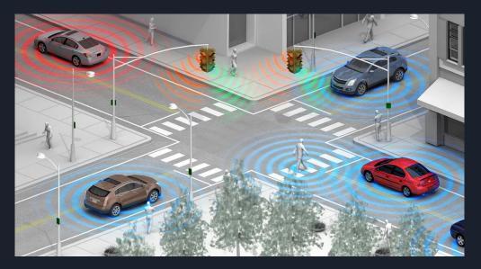
Vehicle-to-vehicle (V2V) communication is communication that enables vehicles to wirelessly exchange information about their speed, location, and heading.
