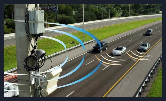
Vehicle-to-Infrastructure (V2I) communication is the wireless exchange of data between vehicles and road infrastructure.
