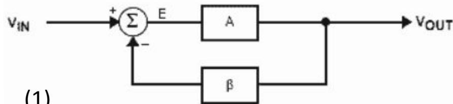
$$V_{OUT} = E \times A \quad (1)$$
