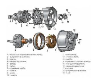
What is called an alternator, an alternator is an electromechanical device that converts mechanical energy into alternating current electrical energy
