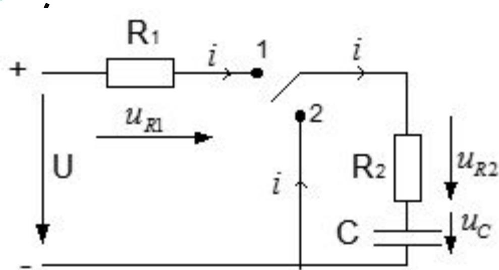
$$u_C = U + Ae^{-\frac{t}{(R_1+R_2)C}}$$
