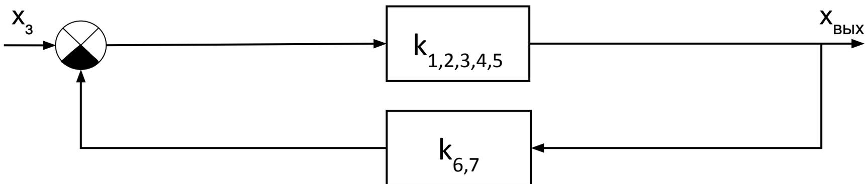
$$X_{\text{ВЫХ}} = \frac{k_{\text{пр}}}{1 + k_{\text{пр}}k_{\text{о.с}}} X_3 = \frac{k_{\text{пр}}}{1 + k_{\text{раз}}} X_3$$
