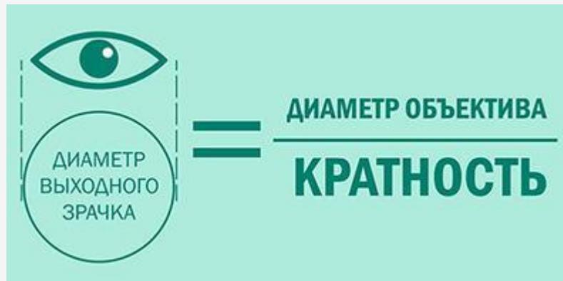
The diagram shows a stylized eye at the top. Below it, a dashed vertical line indicates the diameter of the exit pupil. To the right of this line is an equals sign, followed by a fraction. The numerator of the fraction is 'ДИАМЕТР ОБЪЕКТИВА' (Objective Diameter) and the denominator is 'КРАТНОСТЬ' (Magnification). Below the fraction, the text 'ДИАМЕТР ВЫХОДНОГО ЗРАЧКА' (Exit Pupil Diameter) is written inside a circle.
