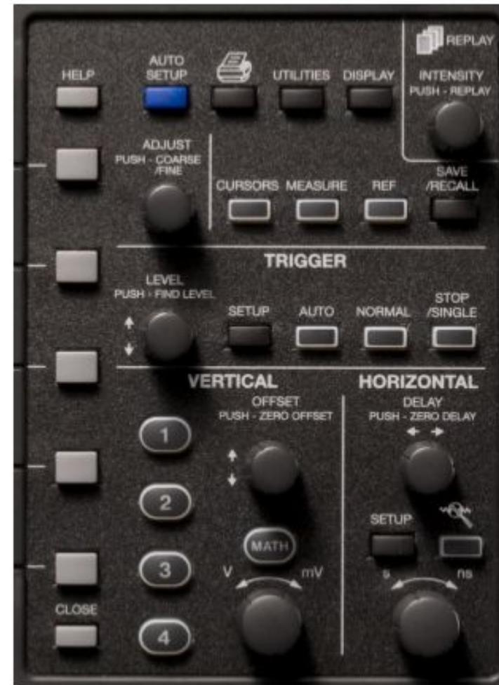
The control buttons of the WaveJet Series front panel are logically grouped into analog and special function areas. The following table provides an explanation of the front panel push buttons and knobs.
