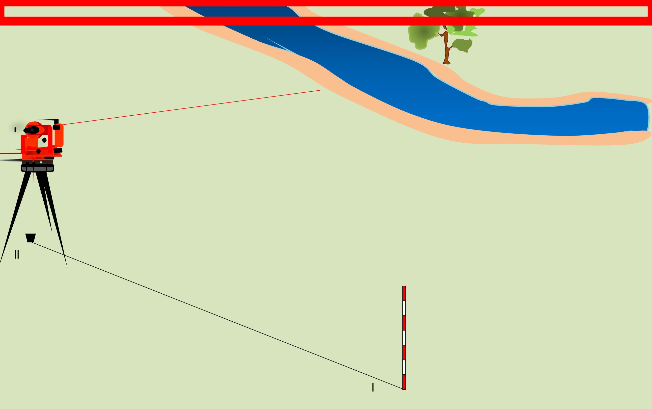
$$\text{Угол } \beta_2 = \text{КЛ1} - \text{КЛ2} = 132^\circ 45' - 62^\circ 25' = 70^\circ 20'$$
