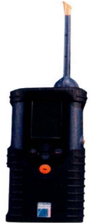
Figure 32.9 The Cyranose 320. The electronic nose may find uses in the food industry, animal husbandry, law enforcement, and medicine. [Courtesy of Cyrano Sciences.]
