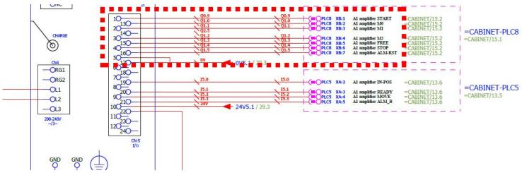
We 'd better assign Ov com for driver input signal ,for all the driver ,in case we use input signal
