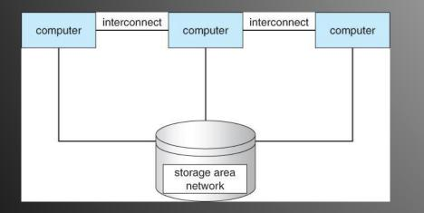
The primitive cluster design itself consists of three computers and a connected network
