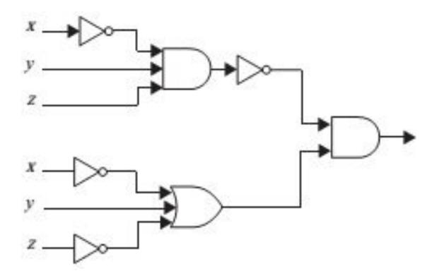
Use K-maps to find simpler circuit with the same output as the circuit shown.
