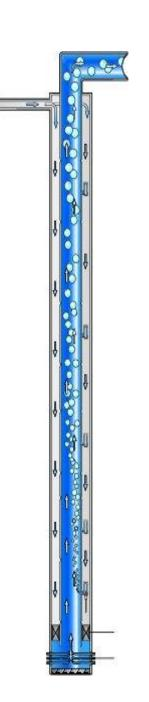
Gas lift is a method of <u>artificial lift</u> that uses an external source of high-pressure gas for supplementing formation gas to lift the well fluids. The principle of gas lift is that gas injected into the tubing reduces the density of the fluids in the tubing, and the bubbles have a "scrubbing" action on the liquids. Both factors act to lower the flowing bottomhole pressure (BHP) at the bottom of the tubing. There are two basic types of gas lift in use today:
