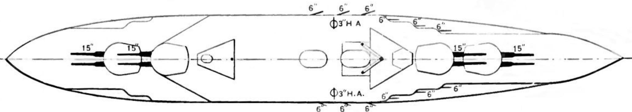
Length, 600 ft. ; 27,500 tons ; Speed, 25 knots ; Completed, 1915-1916 ;
