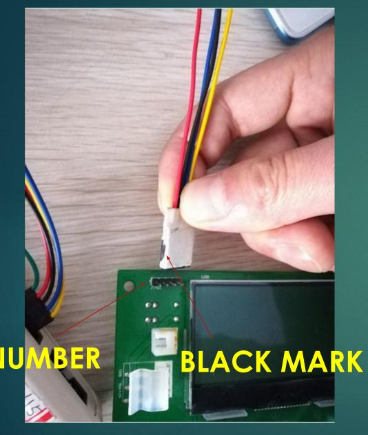
2: CONNECT RECORDER TO PCB,NOTE: KEEP CORRECT POSITION, BLACK MARK SIDE TO NUMBER 1.
