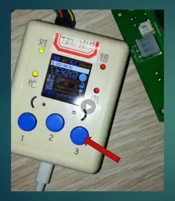
3: PRESS BUTTON 3, THE DISPLAY WILL SHOW "正在烧 写", MEANS "WORKING", WHEN DISPLAY"烧写成功" , IT IS DONE. 4: AFTER RECORD THE PROGRAM, POWER ON PCB AND RESTORE FACTORY DEFAULTS. – POWER OFF AND THEN PRESS AND HOLD THE SETTING BUTTON, POWER ON.
