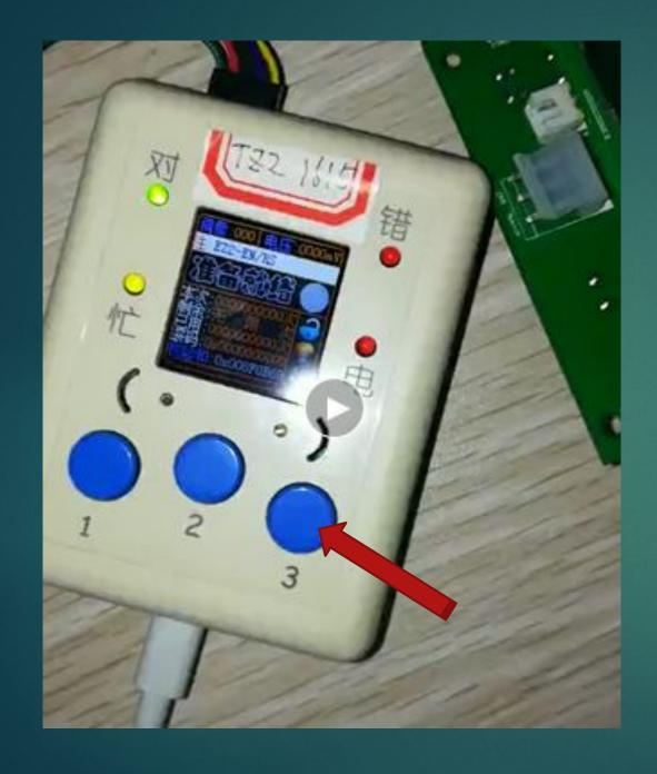
3:PRESS BUTTON 3, THE DISPLAY WILL SHOW "正在烧写", MEANS "WORKING", WHEN DISPLAY"烧写成功", IT IS DONE.
