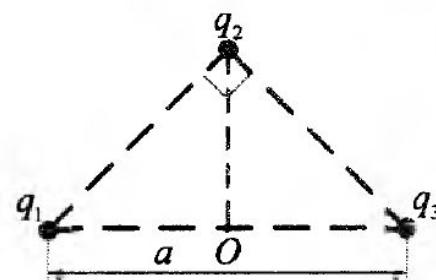
$$\varphi = \varphi_1 + \varphi_2 + \varphi_3 = \frac{kq_1}{0,5a} + \frac{kq_2}{0,5a} + \frac{kq_3}{0,5a} =$$
