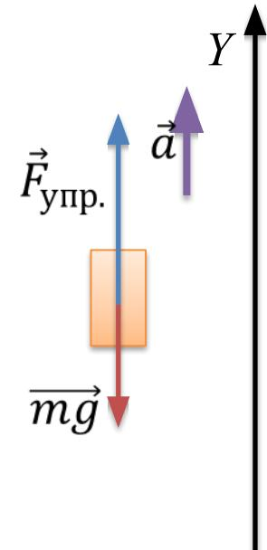
$$\begin{aligned} \Delta l &= \frac{F_{\text{упр.}}}{k} = \frac{m(g + a)}{k} = \frac{0,5(10 + 2)}{25} = \frac{6}{25} = \\ &= 0,24(\text{м}) = 24(\text{см}) \end{aligned}$$
