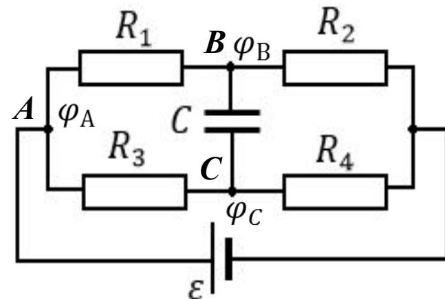
$$U_1, U_3 - ? \quad U_1 = I_{1,2}R_1 = \frac{\mathcal{E}}{R_1 + R_2} \cdot R_1 = \frac{\mathcal{E} \cdot R_0}{4R_0} = \frac{\mathcal{E}}{4} = \frac{160 \text{ В}}{4} = 40 \text{ В}$$
