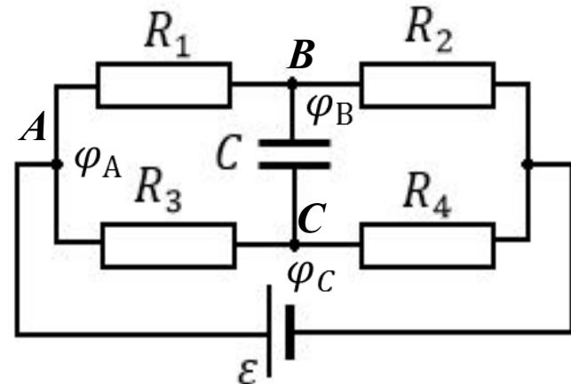
$$U_{CB} = \varphi_C - \varphi_B = \varphi_A - U_3 - (\varphi_A - U_1) = U_1 - U_3$$
