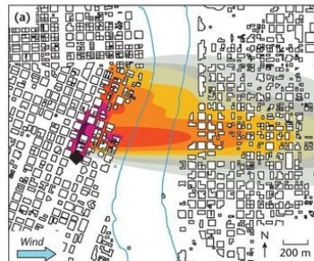
Figure 11.11 Simulated plume dispersion from a hypothetical ground-level source located in central Portland, United States, (a) with and (b) without the effects of buildings near the release incorporated (Modified after Brown, 2004).
