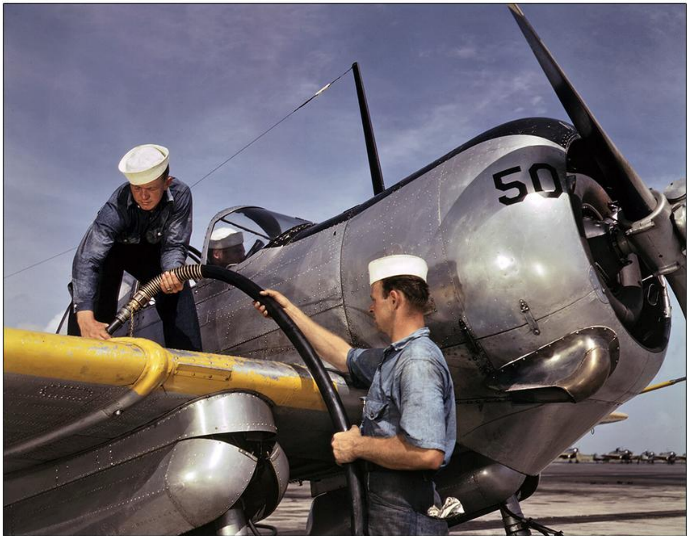
August 1942. "Feeding an SNC advanced training plane its essential supply of gasoline is done by sailor mechanics at the Naval Air Base, Corpus Christi, Texas."
