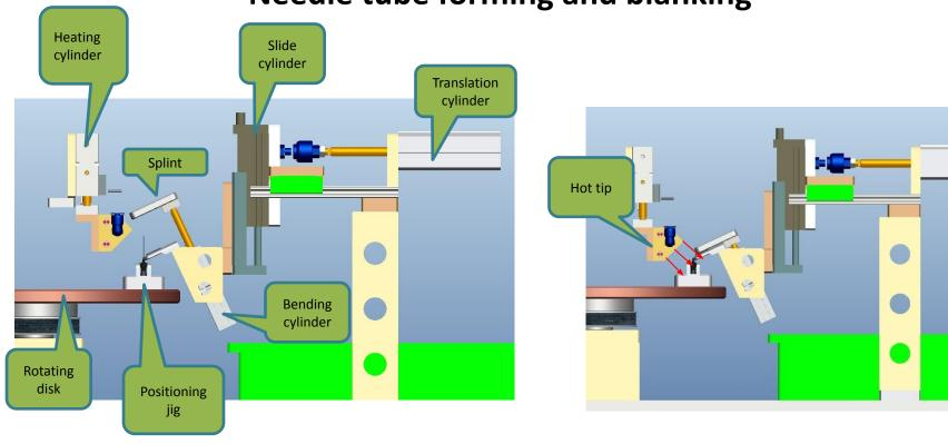
The needle tube is rotated to the forming station, and the cylinder motion splint is moved to the needle tube
