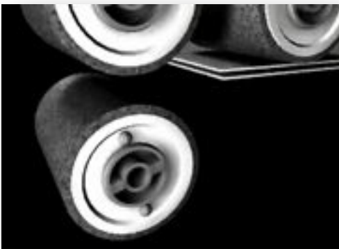
Double sheet push back roller
