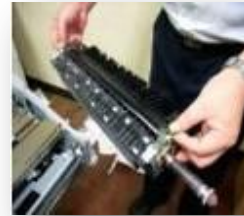
Paper transfer roller unit
