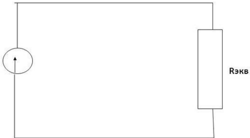
$$I = \frac{E}{R_{\text{экв}} + r} \quad I = 23 \text{ (A)} ; I_1 = I;$$
