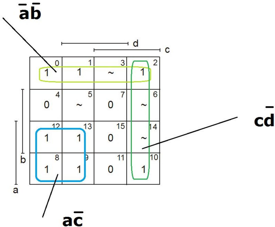
$$f(abcd) = \bar{a}\bar{b} \vee c\bar{d} \vee a\bar{c}$$
