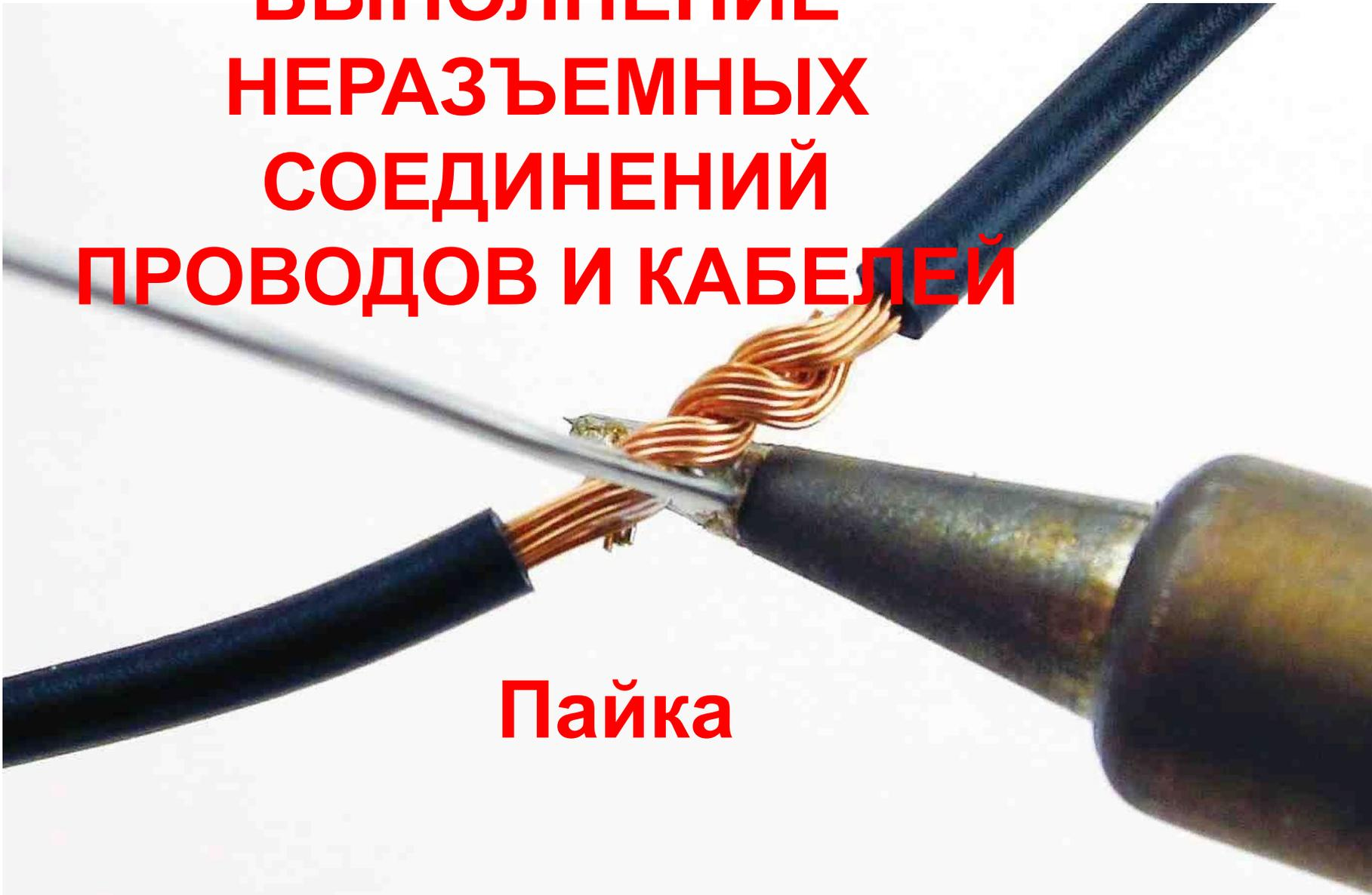
A close-up photograph showing a soldering iron tip being used to join two twisted copper wires. The wires are held together by a small amount of molten solder. The soldering iron has a dark, cylindrical handle and a metal tip. The background is a plain, light color.
