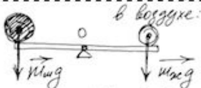
$$F_{\text{тнц}} = m_{\text{ц}}g = \rho_{\text{ц}} V_{\text{ц}} g$$
