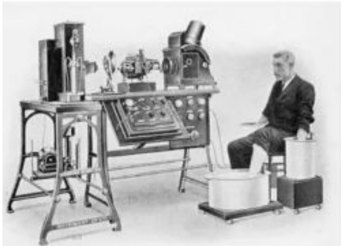
PHOTOGRAPH OF A COMPLETE ELECTROCARDIOGRAPH, SHOWING THE MACHINES BY WHICH THE ELECTRICAL ACTIVITY OF THE PATIENT, IN THIS CASE THE HEART AND THE FOUR BRANCHES OF THE LUNG OF HALL BURTON.
