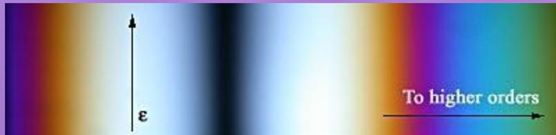
Addition of a quarter wave plate to the quartz wedge with large indices perpendicular. Both retardations subtract. It is possible to find a thickness so that retardation at the center and along directions at  $45^\circ$  of the crystal indices is equal to 0.
