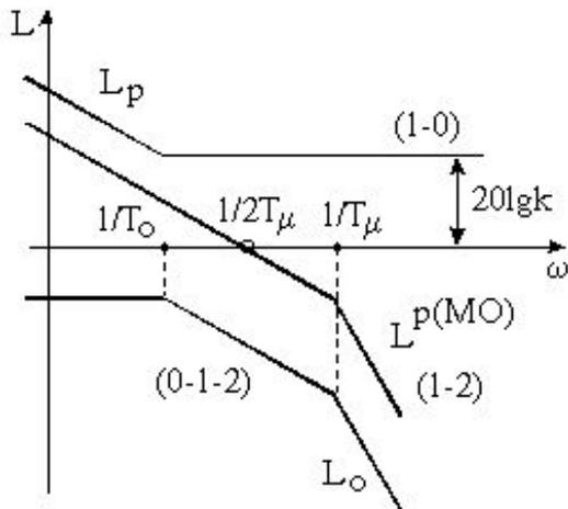
$$W^{P(MO)}(p) = W_p(p)W_o(p) = \frac{1}{2T_\mu p(T_\mu p + 1)}$$
