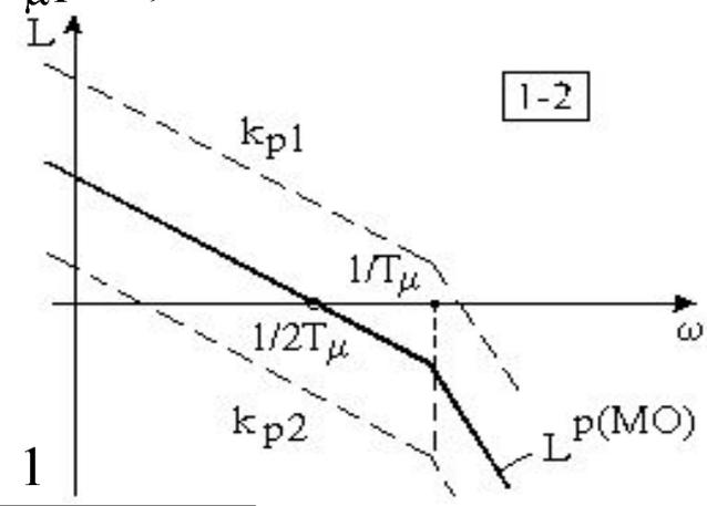
$$W_3^{3(MO)}(p) = \frac{W^{p(MO)}(p)}{1 + W^{p(MO)}(p)} = \frac{\frac{1}{2T_\mu p (T_\mu p + 1)}}{1 + \frac{1}{2T_\mu p (T_\mu p + 1)}} = \frac{1}{1 + 2T_\mu p + 2T_\mu^2 p^2}$$
